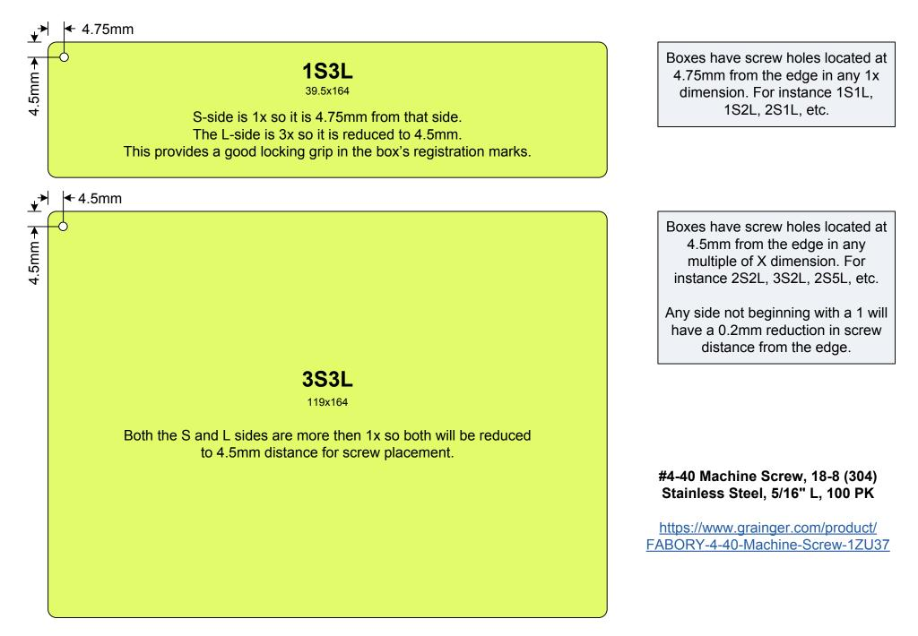
Screws used for registration are #4-40 machine screws with Fillister Head (aka cheese head) and are 5/16" long. They are available for only a couple of bucks per thousand in bulk. They can also be bought in smaller amounts from granger and other online suppliers.
